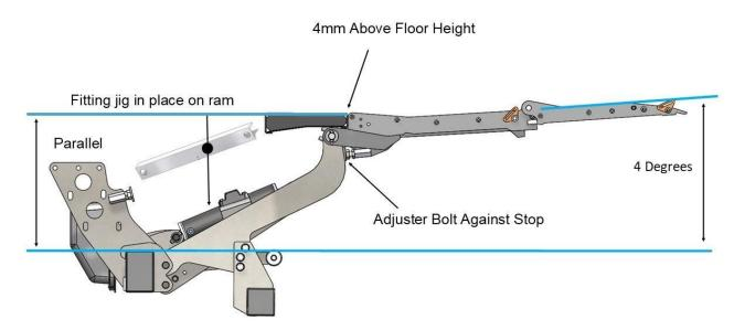
10. When correctly positioned, if the chassis runner is steel, run 3 off 1" long stitch welds around the top of the mounting plate, welding it to the runners on both sides. Also bolt the mounting plate to the chassis with one bolt each side only. If the runner is aluminium or cannot be welded, bolt the mounting plates to the runner and chassis with 3 bolts each side only (ensure a large span of bolts).
