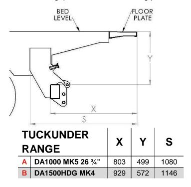
Dimension Y – Distance from the bed of the vehicle to the top of the tailift beam, reference only.
