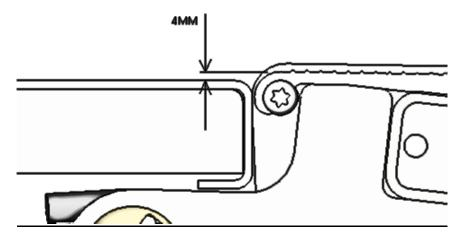
Swing the tailift beam under the vehicle body, so that the mounting plates fit either side of the chassis. Ensure that the lift is positioned central about the chassis. If the gap between the mounting plates and the chassis exceeds 2mm each side, a shim should be inserted between the mounting plate and the chassis. Using a trolley jack, adjust the position of the beam ensuring that the top of the beam is parallel with the floor of the vehicle.
