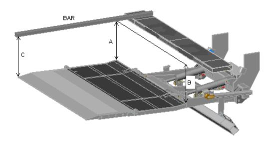
Apply a load equal to the safe working load +25% to the platform, leave it for a few seconds before removing it (note that the power pack relief valve prevents this load from being lifted).
