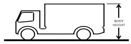
Note that the lift can be used to tip into the side of the body, in these cases the 'body height' dimension will be from the ground to the bottom of the hole in the side of the body, into which the bin will tip.
