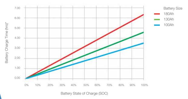
\* Charge time based on 1.5kW charger @ 15° C Ambient
