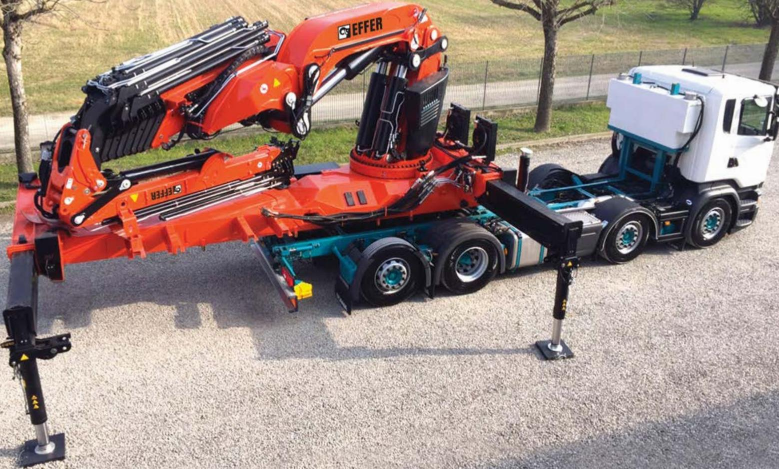
The 2055 crane combines the main technological Effer innovations both from a technical-structural point of view and in terms of safety, because it is equipped with the PROGRESS electronic control system.
