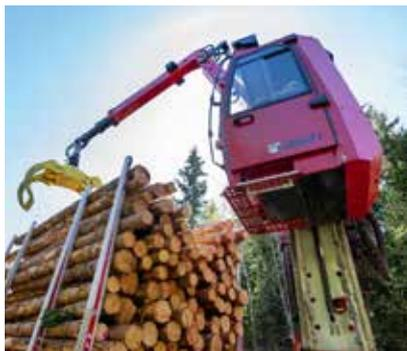
**High Seat** offers both standard mechanical crane controls and a cutting-edge electric joystick with an intuitive user interface that delivers smooth operation and precision. Featuring a refined safety system, High Seat is ergonomic, heated and weather-resistant, and it's easy to position since its fully adjustable.
