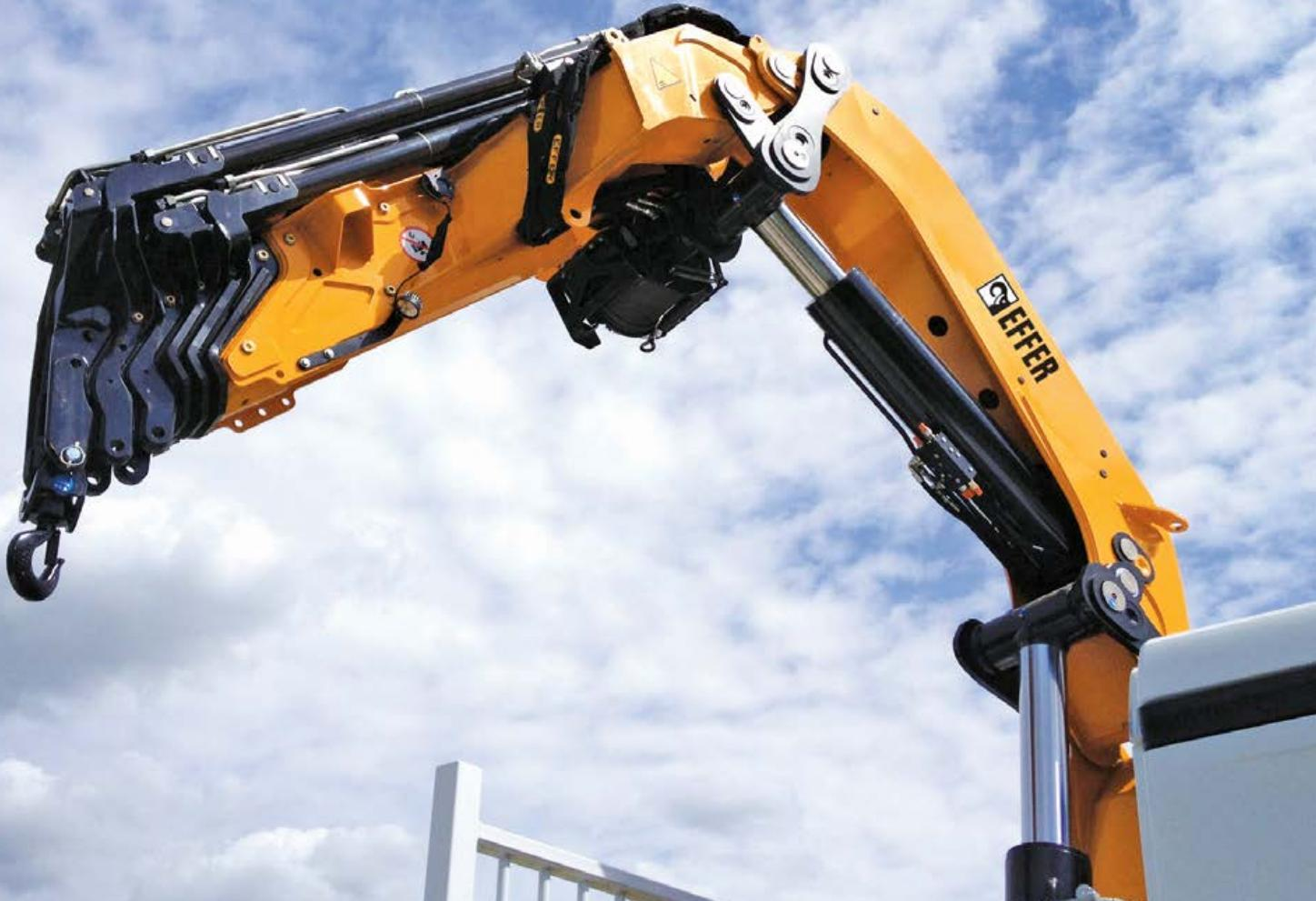
The 525 crane may be considered the ultimate expression of the lifting moment/weight ratio in the whole category. The use of materials with very high structural strength, the electronics, the advanced design systems and the possibility to use powerful and light joints, allow the crane to achieve the dual concept of lifting capacity and operating speed. The introduction of the PROGRESS electronic system has also made it possible to reach the highest safety standards.
